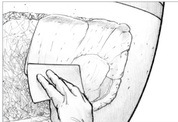
Figure 4-12 Apply a layer of epoxy/406 thickened to a mayonnaise consistency.
