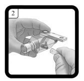
2. Attach other end of Pressure Tube to Nipple on Air Connector # 3. NOTE: Air Pressure Tube # 8 has a one-way Check Valve installed. The airflow direction must be from Air Connector towards the Pressure Pot. The tapered side of the Check Valve must point towards the pressure pot.
