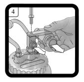
4. Secure Air Connector Bracket to Fluid Coupler by inserting the threaded end of the Hook # 1. Tighten locking nut # 2. Both Fluid Coupler and Air Hose Outlet of the Air Connector must be pointing toward the same direction after installation is complete.
